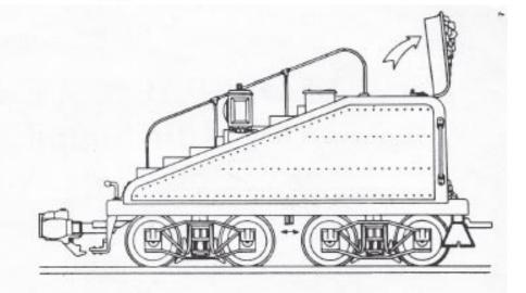
Remove the coupler on the locomotive and connect the tender connection coupler with 2.3 x 6 screw provided.
